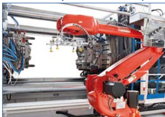
KW 2000 - Four injection units and a rotary table.
